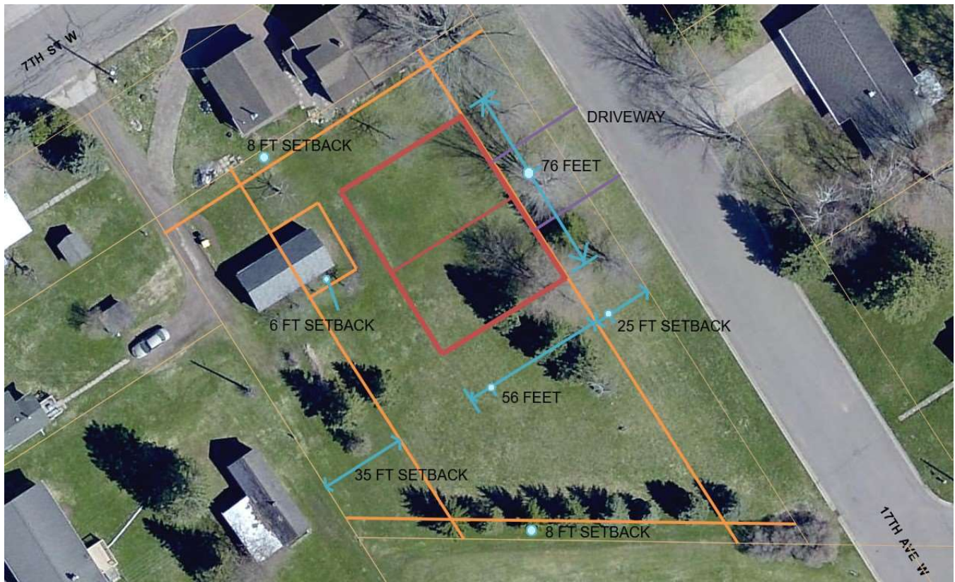
Aerial photo of the site depicting the location of buildings and setbacks
