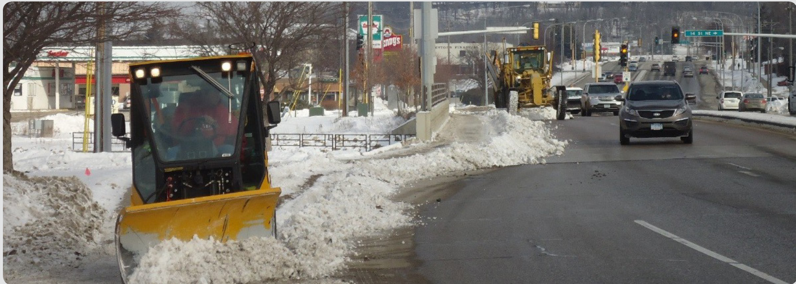
Figure 8: A City of Rochester employee clears a sidewalk with a Trackless tractor (left). Credit: City of Rochester
