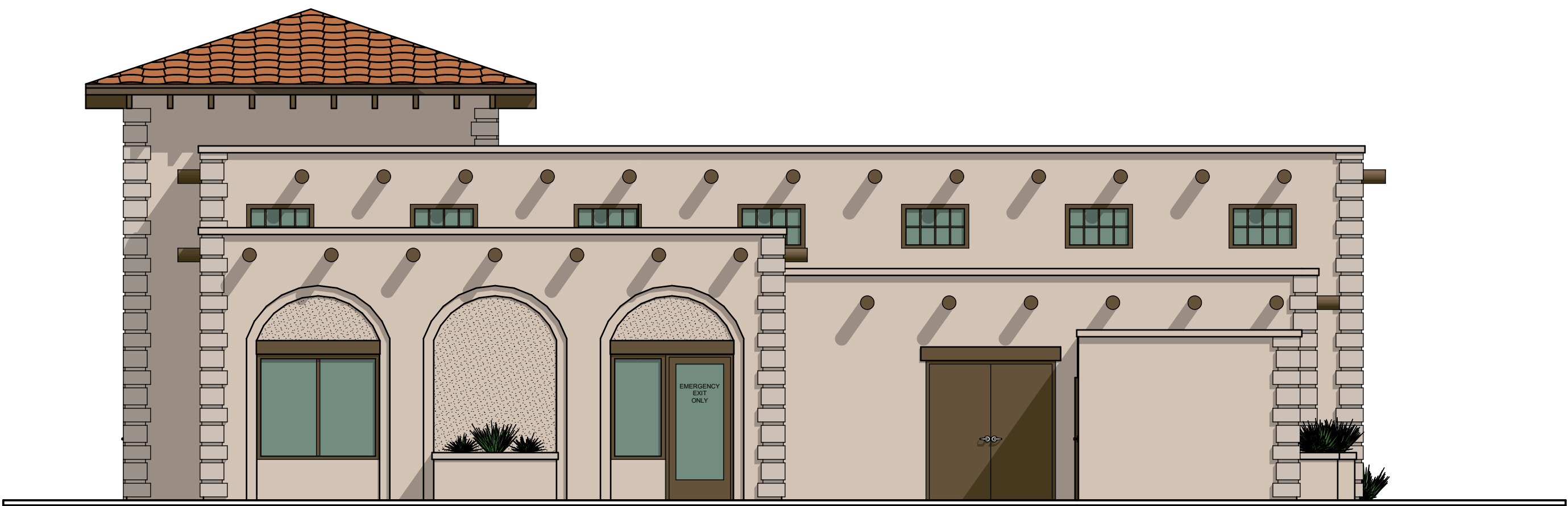
EAST ELEVATION (DELIVERY SIDE) SCALE: 3/16" = 1'-0"
